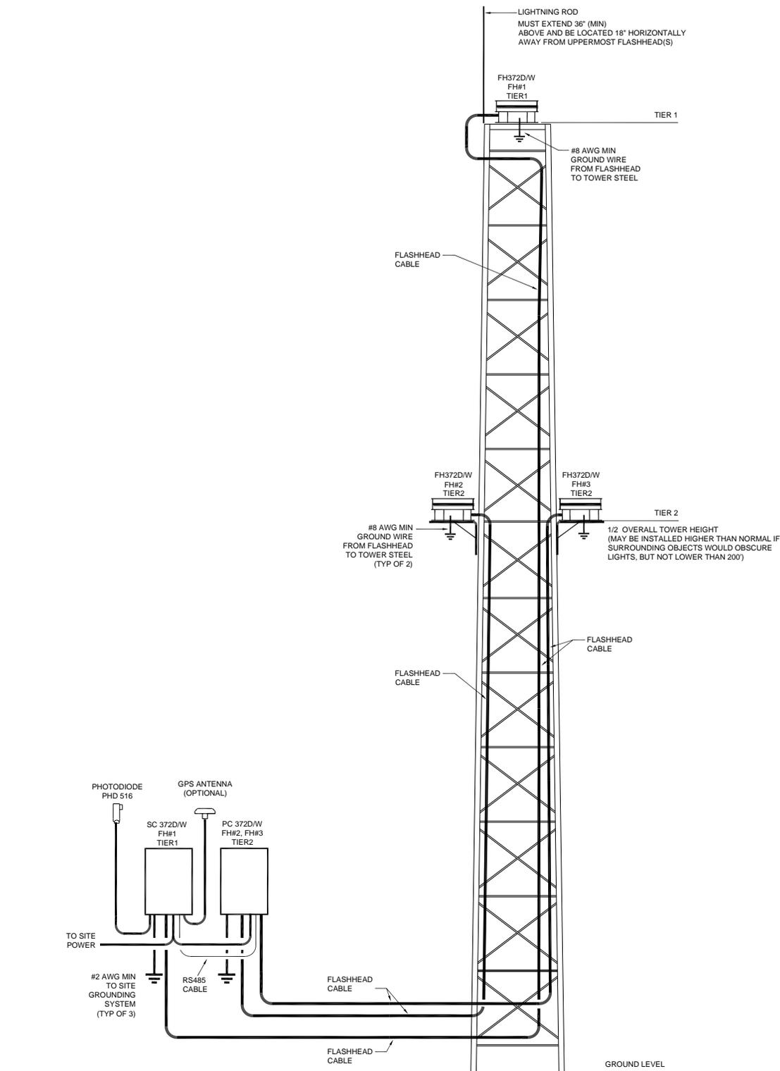
Figure 2-20 – Typical E2/D2 Avian Component Locations (AC 70/7460-1M)
