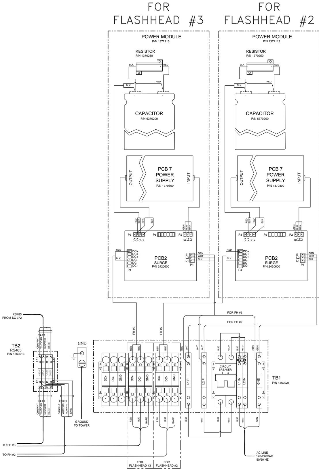
Figure 2-38 – PC 372 (AC) Internal Wiring for E2, D2
