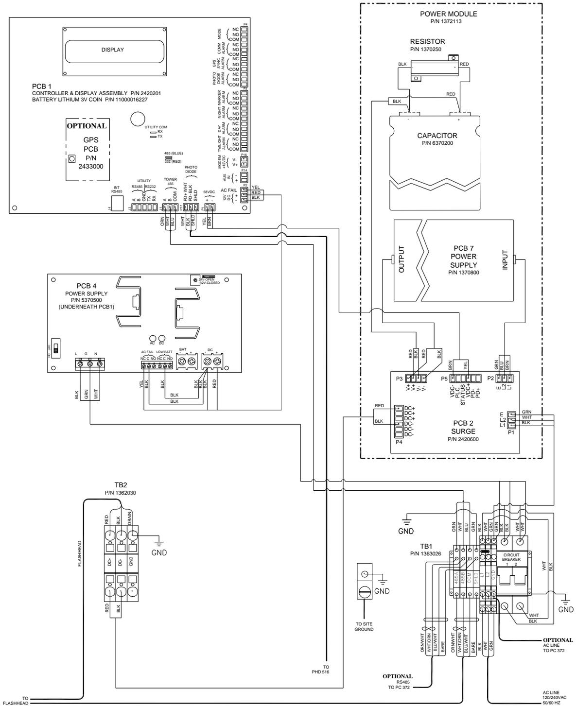
Figure 2-33 – SC 372 (AC) Internal Wiring
