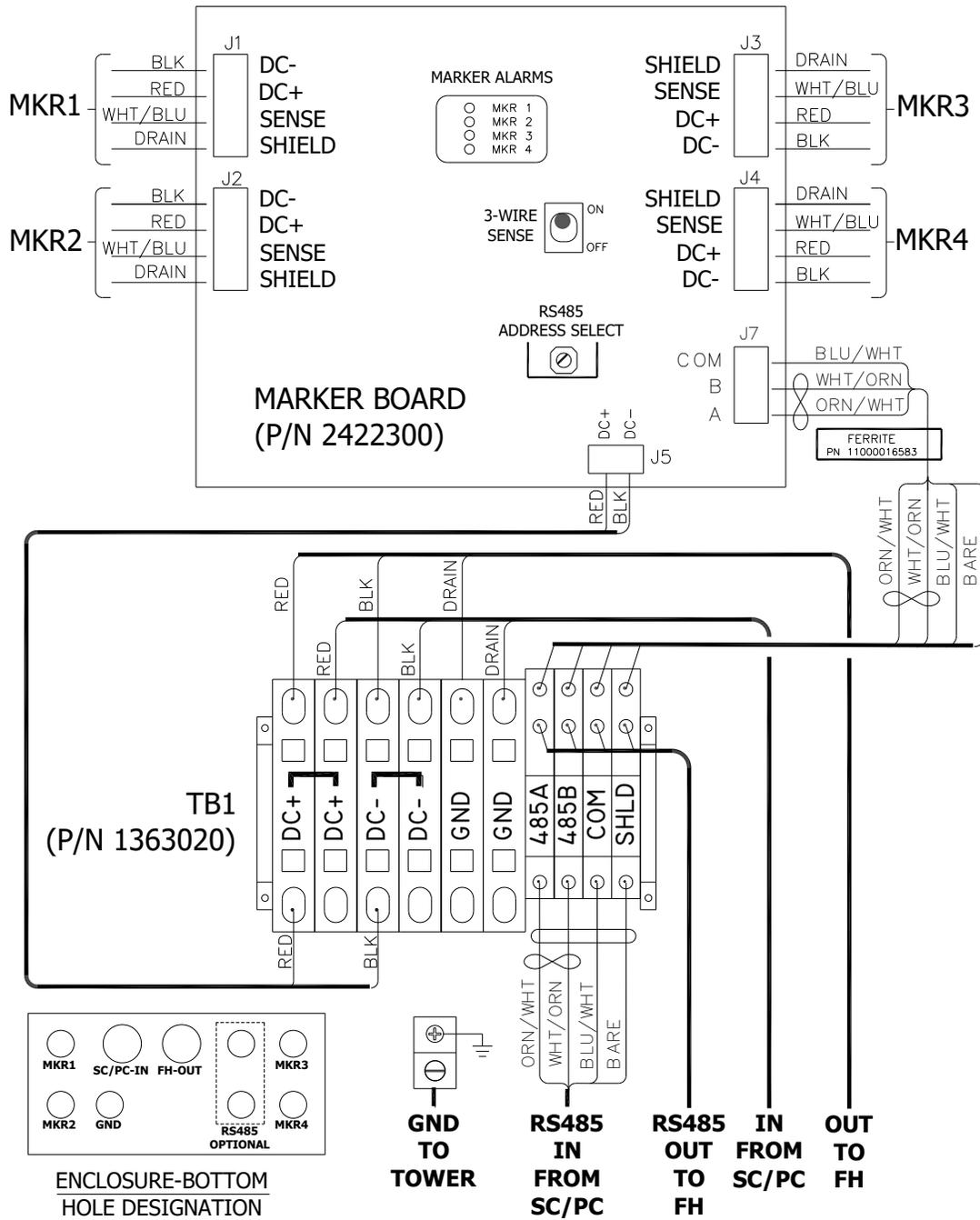
Figure 2-40 – Marker Interface Wiring Diagram
