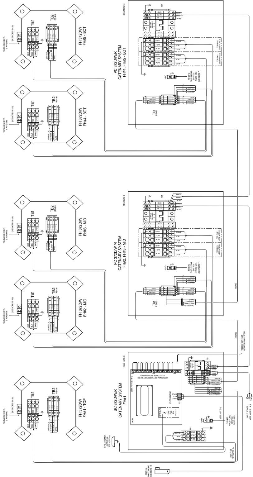
Figure 2-31 – Typical Catenary System Wiring Diagram (With 5 Lights)
