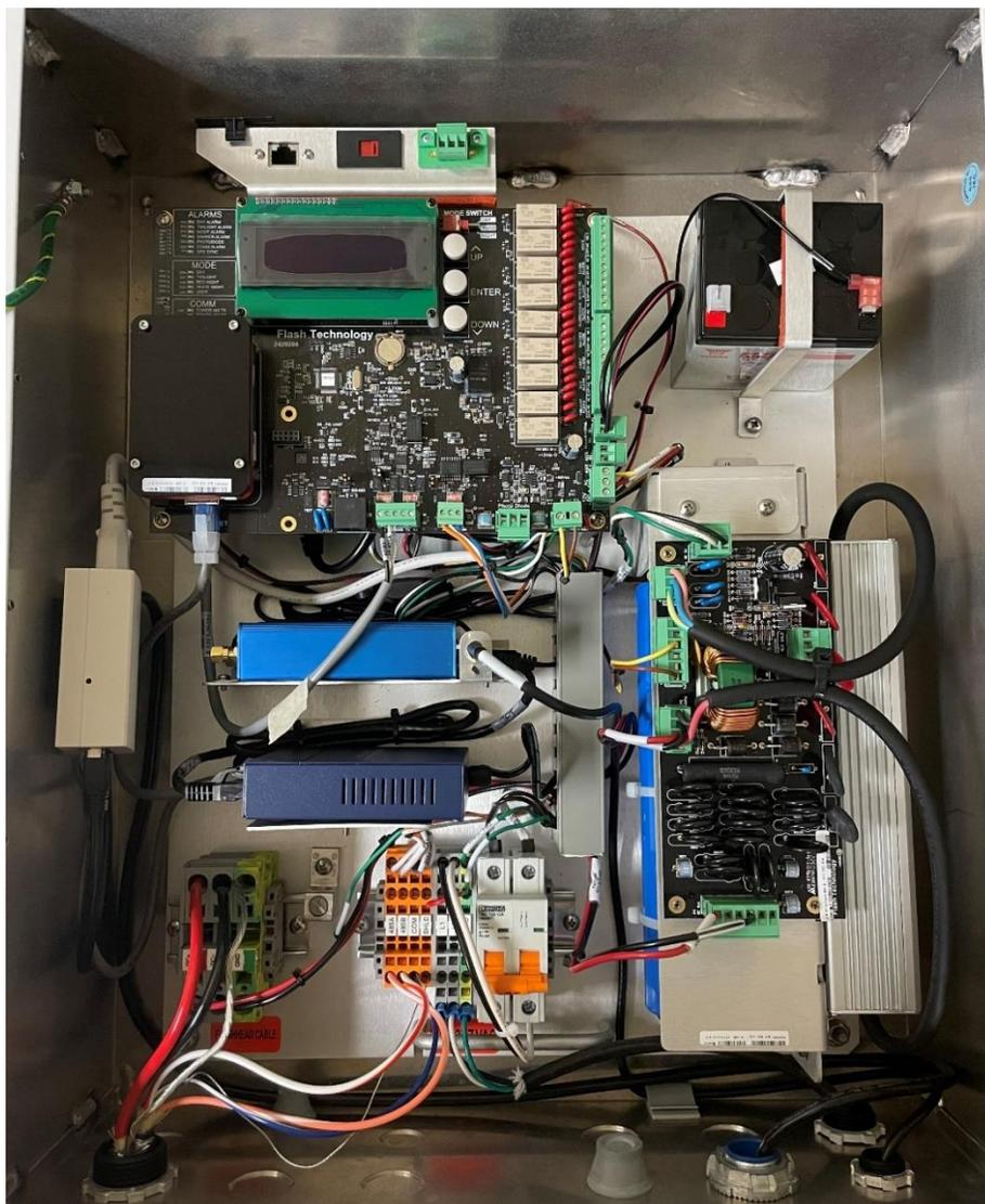
**Note:** Shows a fully loaded unit with optional modem, Wi-Fi and generator monitoring kits.
