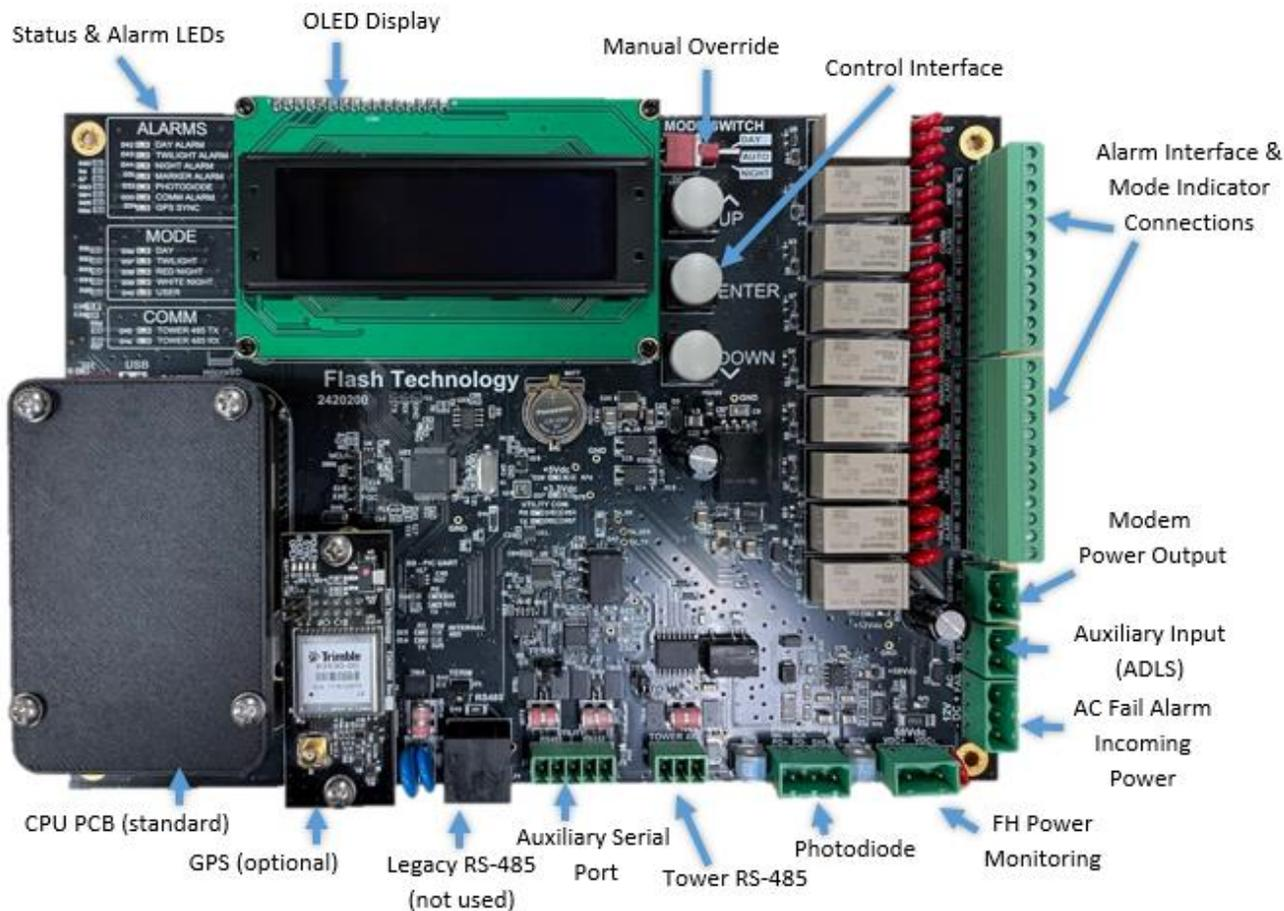
Figure 1-2 – PCB1 Controller Board
