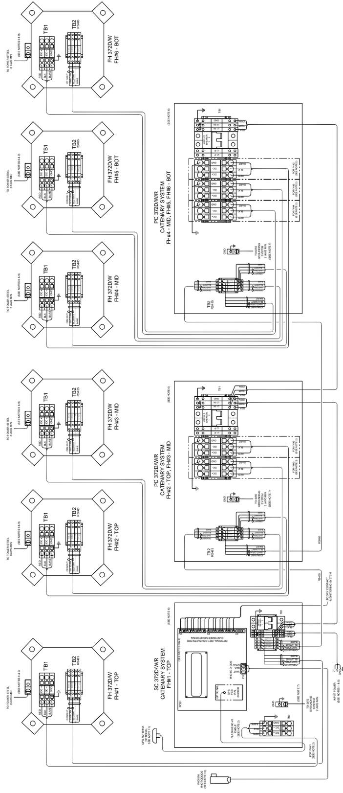
Figure 2-32 – Typical Catenary System Wiring Diagram (With 6 Lights)
