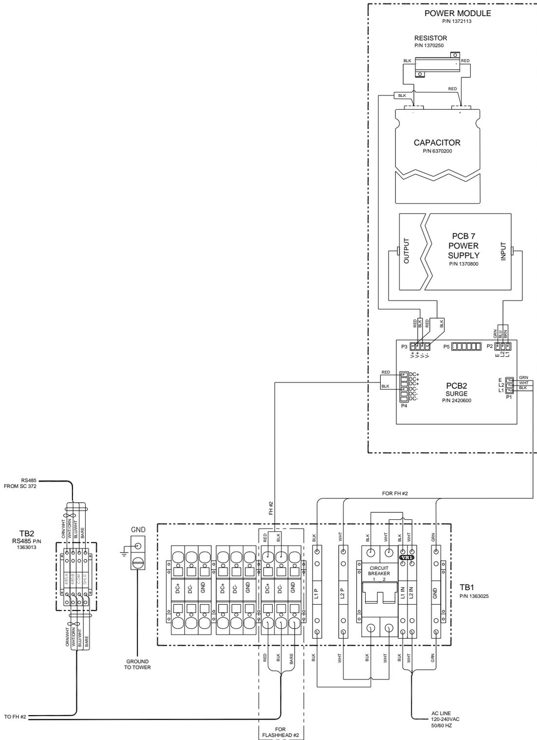
Figure 2-37 – PC 372 (AC) Internal Wiring for E1+1, D1+1
