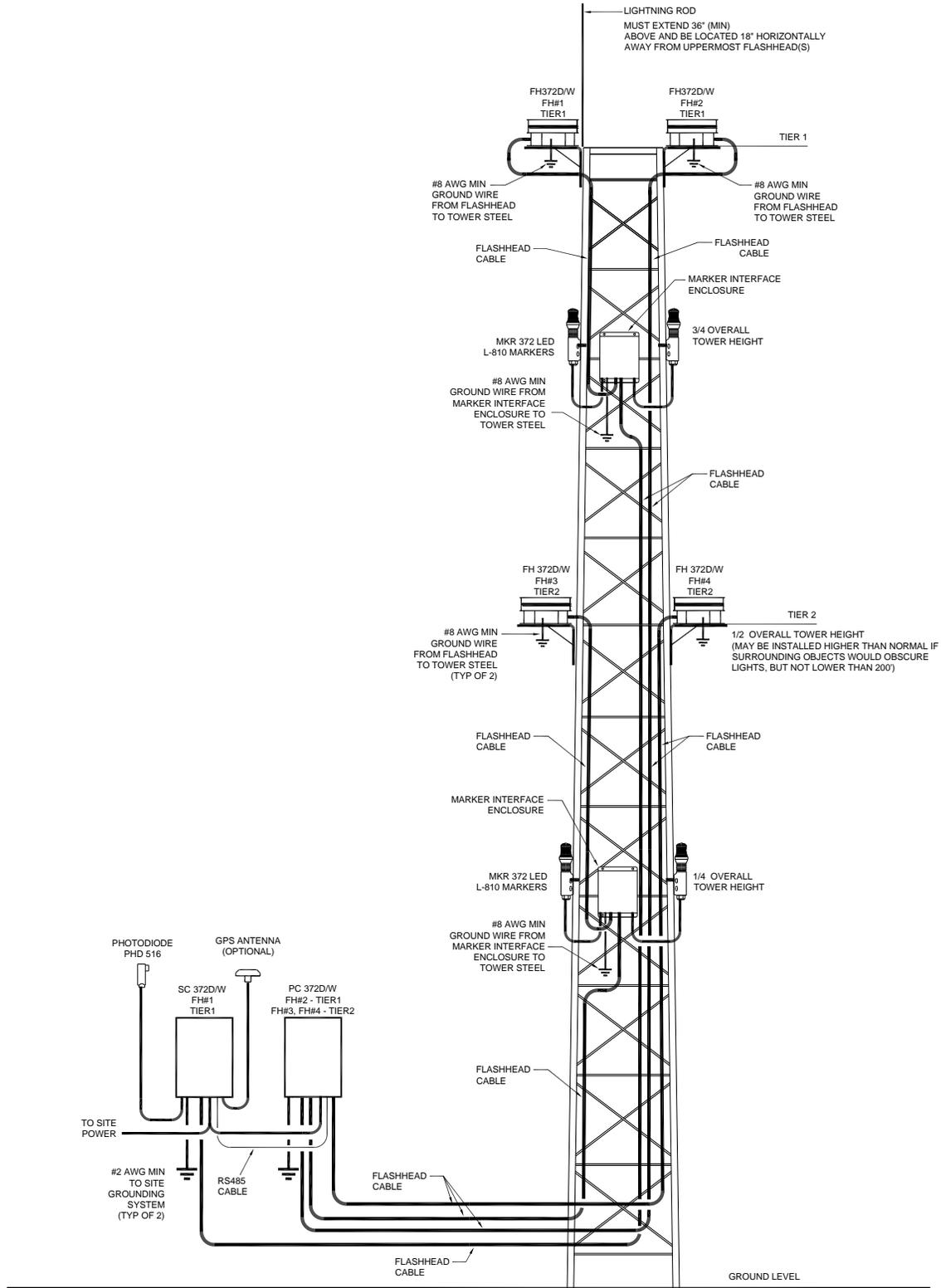
Figure 2-21 – Typical E2+1 Component Locations (AC 70/7460-1M)
