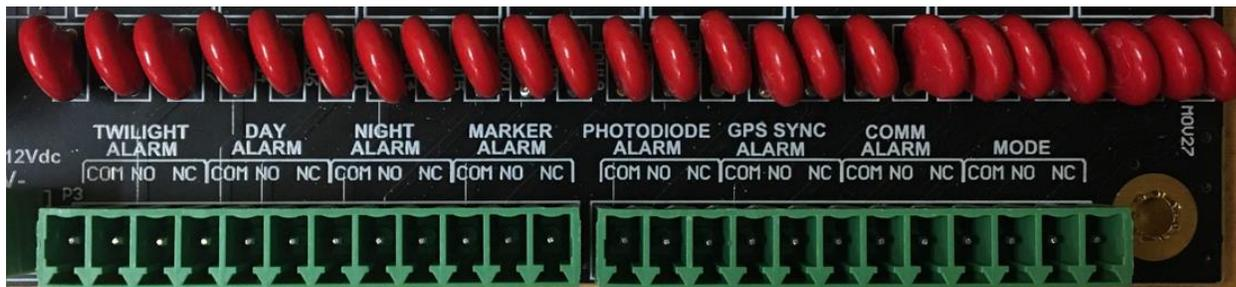
**Figure 1-4 – Alarm Interface and Mode Indicator Connections**
