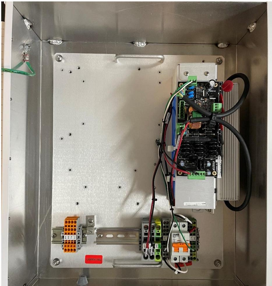
Figure 1-6 – PC 372 Power Converter in E1+1 configuration (1 power supply modules)
