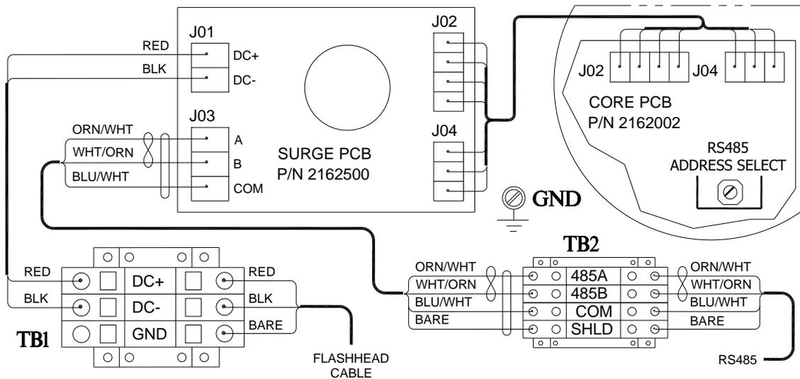
Figure 2-41 – FH 372 Wiring Diagram
