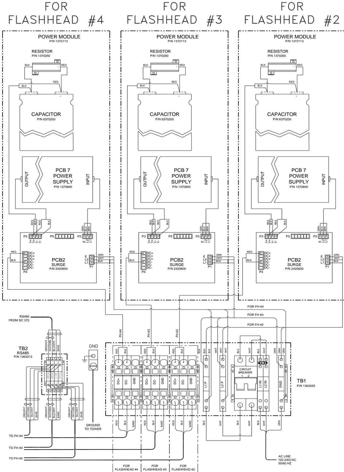
Figure 2-39 – PC 372 (AC) Internal Wiring for E2+1, D2+1
