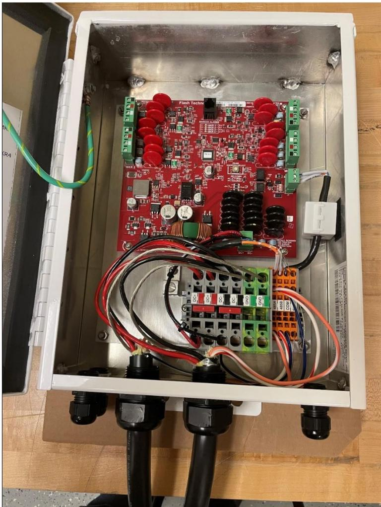
Figure 2-6 – Marker Interface Box and Wiring
