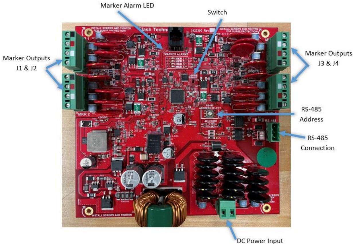
Figure 1-8 – Marker Interface PCB
