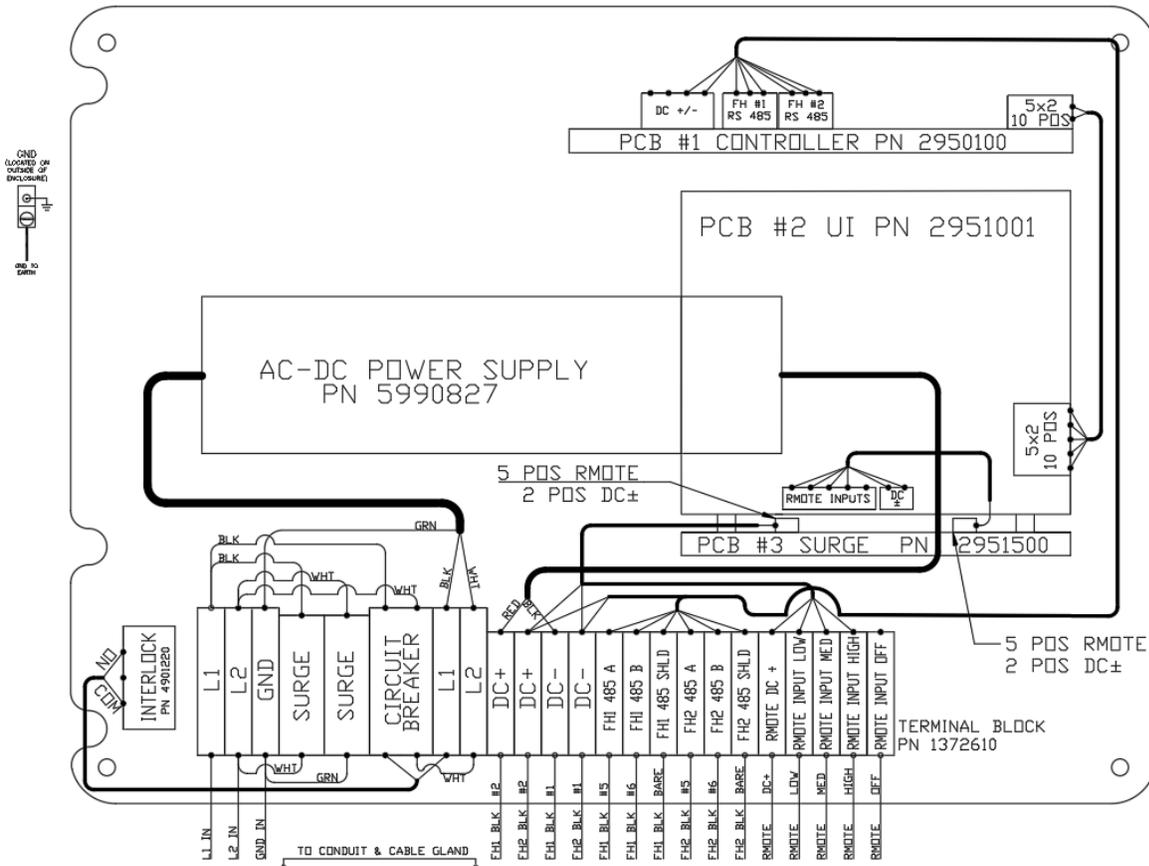
**Figure 2.4 – System Wiring Diagram**
