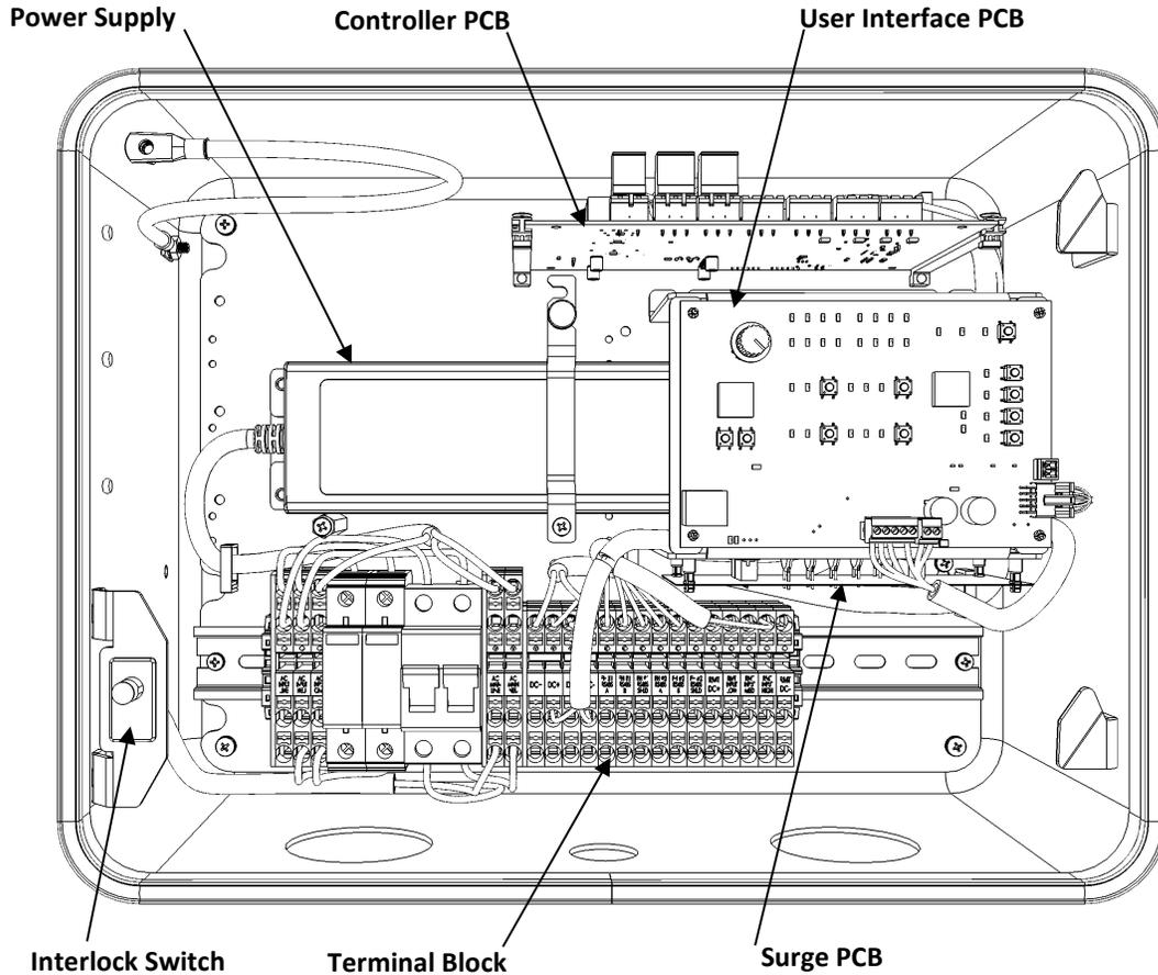
Figure 1.2 – PC 800(L) Internal Components
