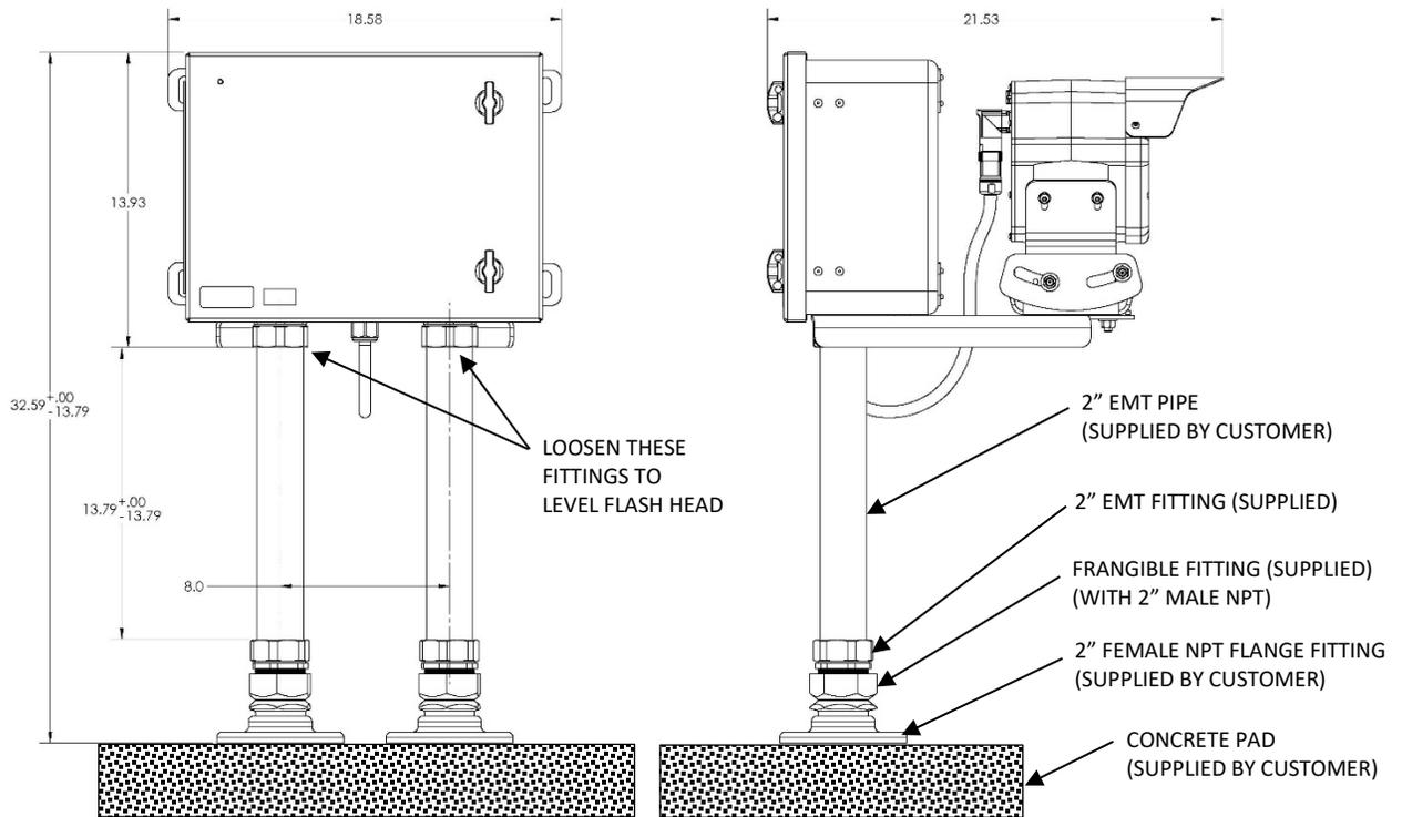
Figure 2.2 – System Dimensions and Mounting Details
