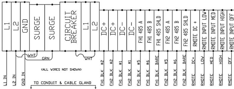
**Figure 2.3 – System Input Wiring**
