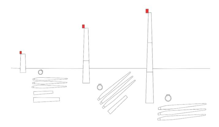
= L-810 (red/infrared side light) Configured to flash in sync with L-864 at 30 fpm
