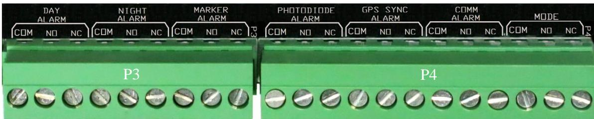
Figure 1-4 – Alarm Interface & Mode Indicator Connections
