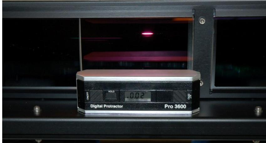
*LHA with the digital inclinometer in place*
