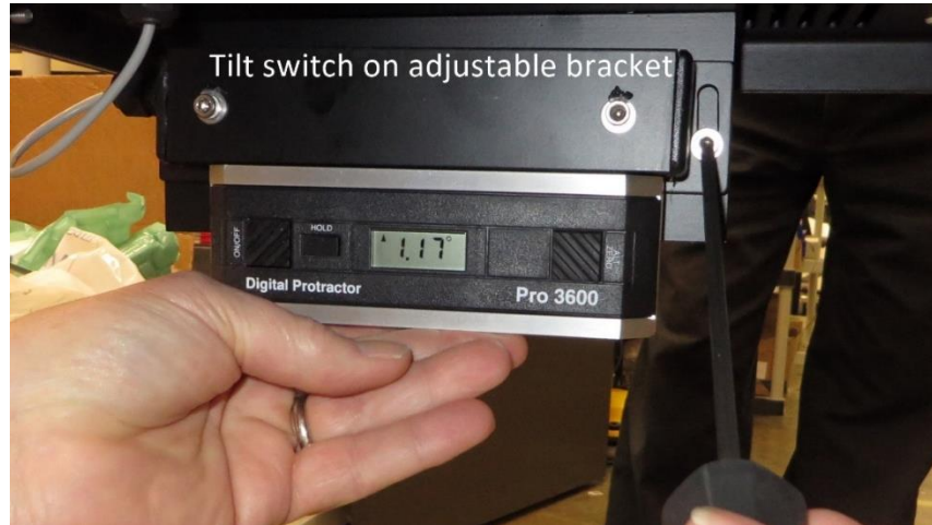
Figure 15: Tilt switch bracket detail
