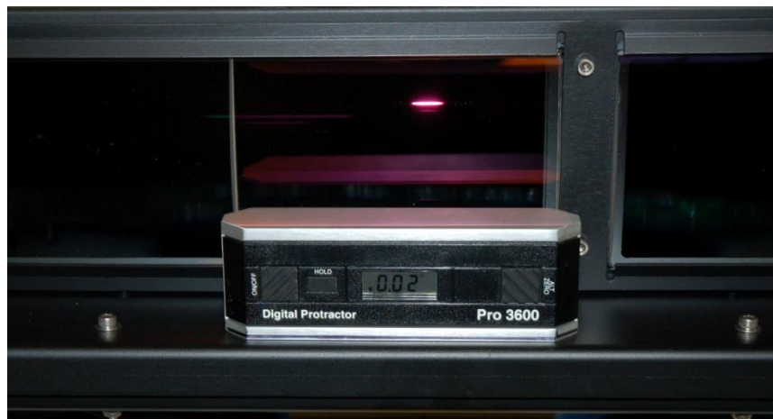
Figure 13: LHA with the digital inclinometer in place
