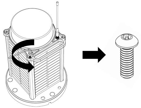
2. Install  $\frac{1}{4}$ -20 screw with tapped hole using provided  $\frac{1}{8}$  hex key. Tighten firmly.
