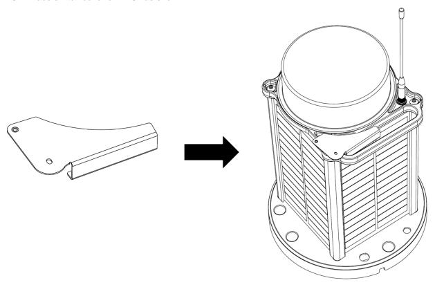
4. Push cover into place so bottom flange slides under A704 top plate as shown.
