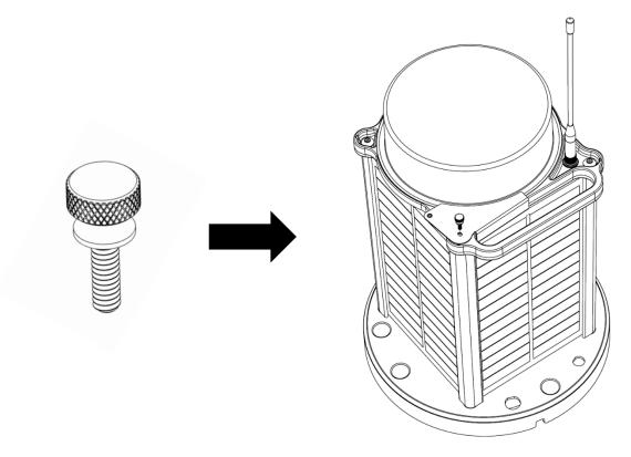
6. When removing the switch cover to access the pushbutton, thread the thumbscrew into the nut insert on the cover to avoid losing it.
