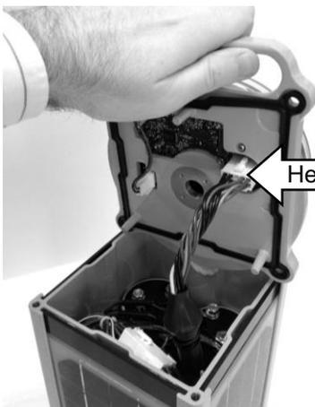
8. Connect the free end of the harness to head connector. The indicator LEDs will light and then start blinking.
