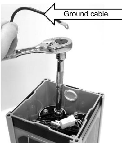
5. Using a 1/2 in. hex socket, remove the battery retention bolt holding down the ground cable. Remove the ground cable and recycle. Reinstall the battery retention bolt and hardware; tighten to 200 in. lbs.
