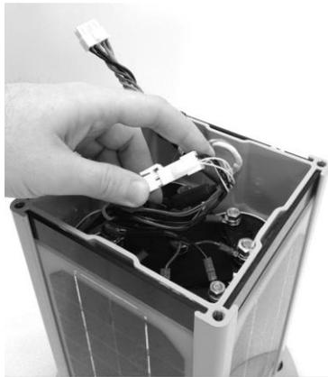
7. Reconnect the battery harness and press together until it is latched.
