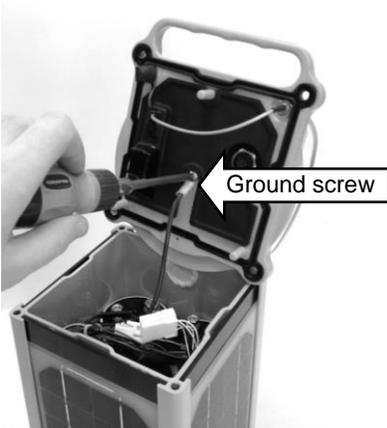
4. Using a #2 Phillips screwdriver, remove the ground screw from the top of the head. This screw can be recycled since it will no longer be used with the new head.
