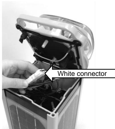
2. Lift off the head by the handle and disconnect the white connector by pressing the latch and pulling apart.
