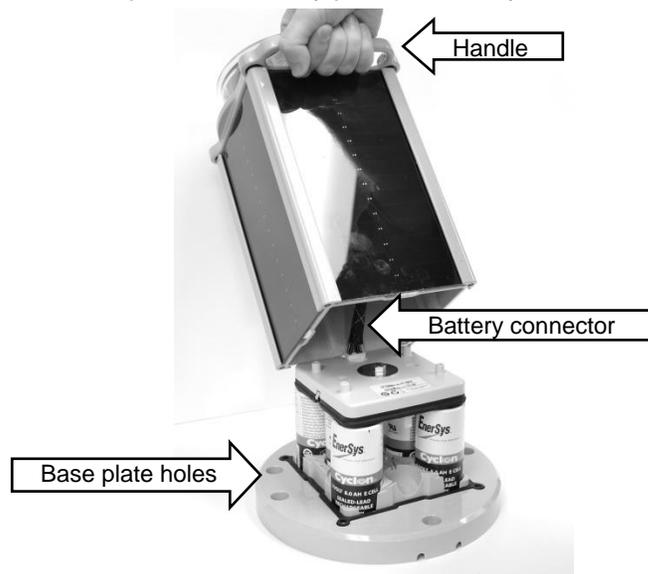
7. Tighten four base plate screws to 40 in.-lbs.
