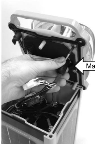
3. Remove the main head connector by pressing on the two raised sides and pulling straight apart.
