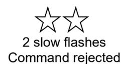
The number symbol # represents 0 - 9. Commands can be rejected if they are unsupported, contain an incorrect key sequence or have an effective intensity too high for the programmed flash code.
