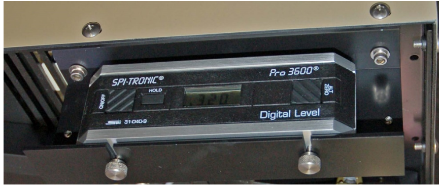
Figure 14: Inclinometer inserted in mounting bracket on the bottom of the LHA
