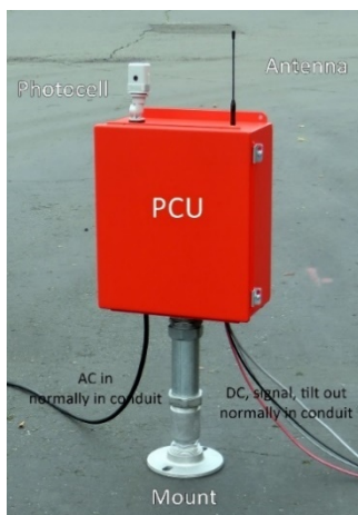
Figure 10: PCU with pre-wired connections (note: shown with a photocell and antenna)
