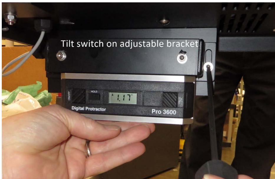
Figure 15: Tilt switch bracket detail
