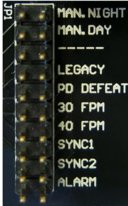
Figure 3-2 – Configuration Jumpers
