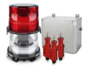
The FTB 324 is an L-864/L-865 system that includes a white xenon flashing light for day, a red xenon flashing light for night and 3 LED markers for structures between 200' and 700' AGL (FAA tower type E1-E2).
