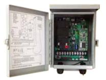
The FTW 170/170-2 wireless synchronization unit supplies a timing pulse to synchronize flashing obstruction lighting on any number of controllers/power converters manufactured by Flash Technology. The structures needing synchronization can be any distance apart without limit.
