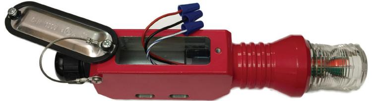
2. Feed the marker cable through the black cord grip and strip approximately 1/4" from the jacket of each conductor. Cut off the the bare drain wire as this will not be used in the marker base.
