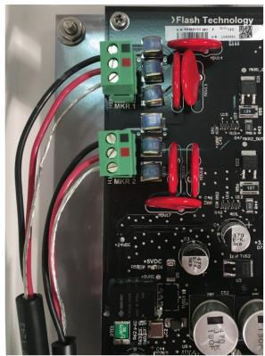
NOTE!! If using V3.4 Firmware or above the markers can be connected to any of the (4) outputs on the board.
