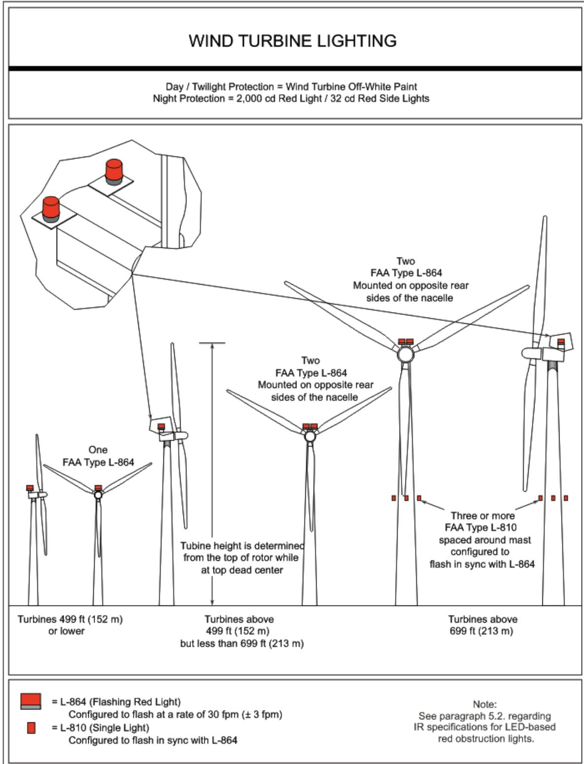
**Figure A-26. Wind Turbine Lighting**
