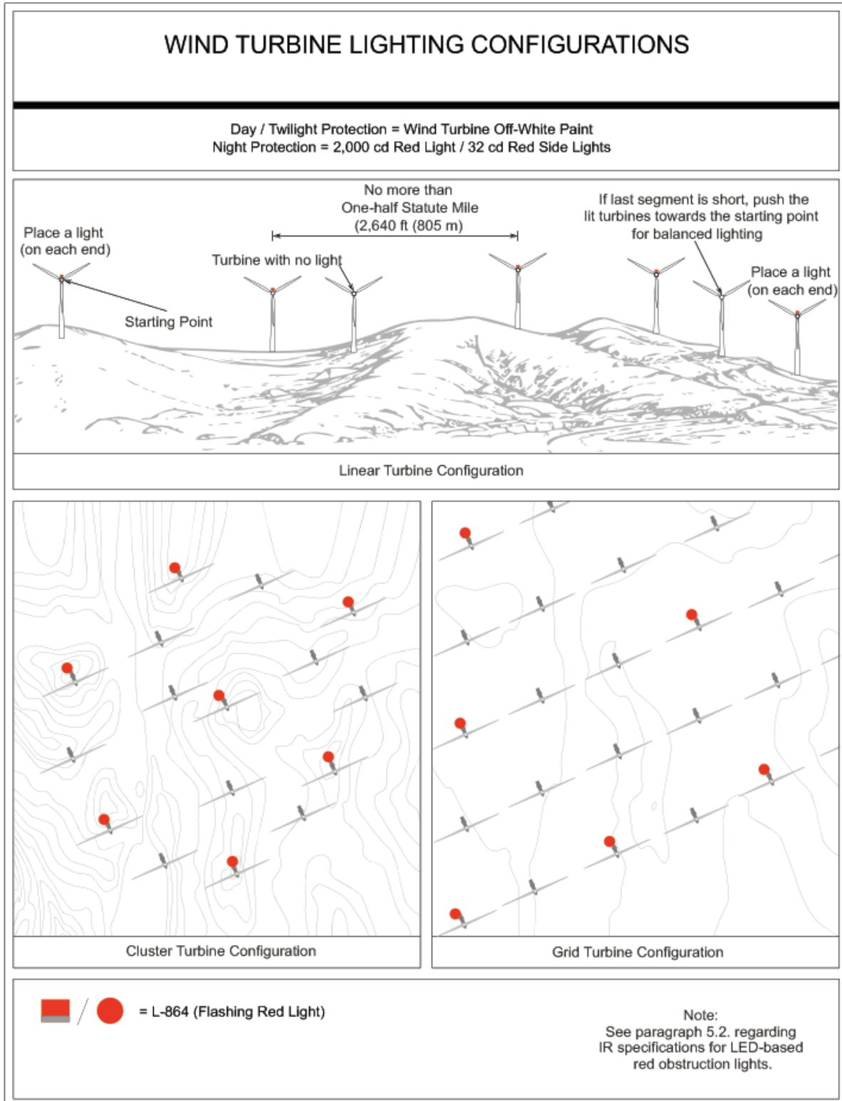
**Figure A-29. Wind Turbine Lighting Configurations**
