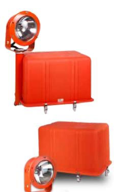
The FTS 830 is a current-driven unidirectional approach light that identifies runway end or the acquisition of an active runway. It can be used as a simple runway end identifier light (REIL) or as an addition to complete any number of approach light systems like MALSR, MALSF, SSALSR, ALSF I and II for runway alignment and runway threshold marking.
