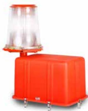
The FTS 400 is a voltage-driven omnidirectional approach light that identifies runway end or the acquisition of an active runway. It can be used as a simple runway end identifier light (*REIL*) or complete omnidirectional approach lighting system for runway alignment and runway threshold marking.
