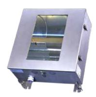
The FTB 205 is an FAA type L-856 high intensity white xenon strobe system that provides white flashing lights for day, twilight and night for structures over 500' AGL (FAA tower types B3-B6 and C3-C6).
