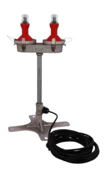
The OL2 mounting bracket is designed to adapt a 3/4" NPT OL2 mount to an available flashhead mounting plate on top of the tower. It elevates the double L-810 unit 12" above appurtenances, providing 360-degree visibility and ensuring an unobstructed view per FAA AC 70/7460.
