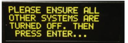
5. After the additional controllers are turned off, verify their outgoing DC voltage is below 5 VDC on the flash head terminal block, and then press “Enter”.
