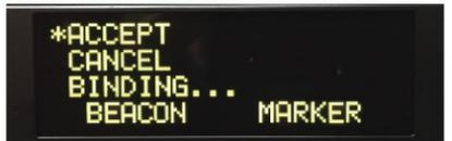
BEACON = LED Beacon (L864/L865) | MARKER = LED Marker J-Box (L810)
