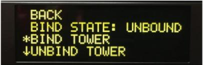
4. If multiple system controllers are onsite, only turn on the unit being bound while following this process.
