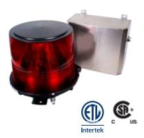
Designed to meet FAA L-864 obstruction lighting requirements, the FTB 302r system includes a high intensity red xenon flashing beacon for night. It is suitable for structures taller than 150' AGL (FAA tower types A1-A6), where a red flashing beacon is needed to complement a high intensity system. The system utilizes the FTC 121 controller.
