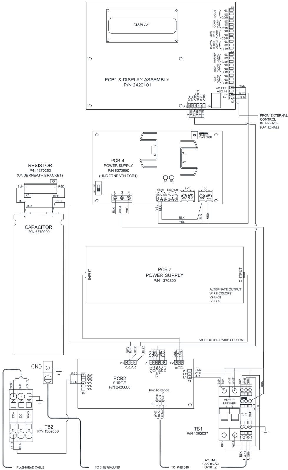
Figure 2-24 – SC 370 (AC) Internal Wiring Standard System
