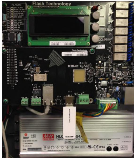
Figure 2-4 – USB Wi-Fi Installation
