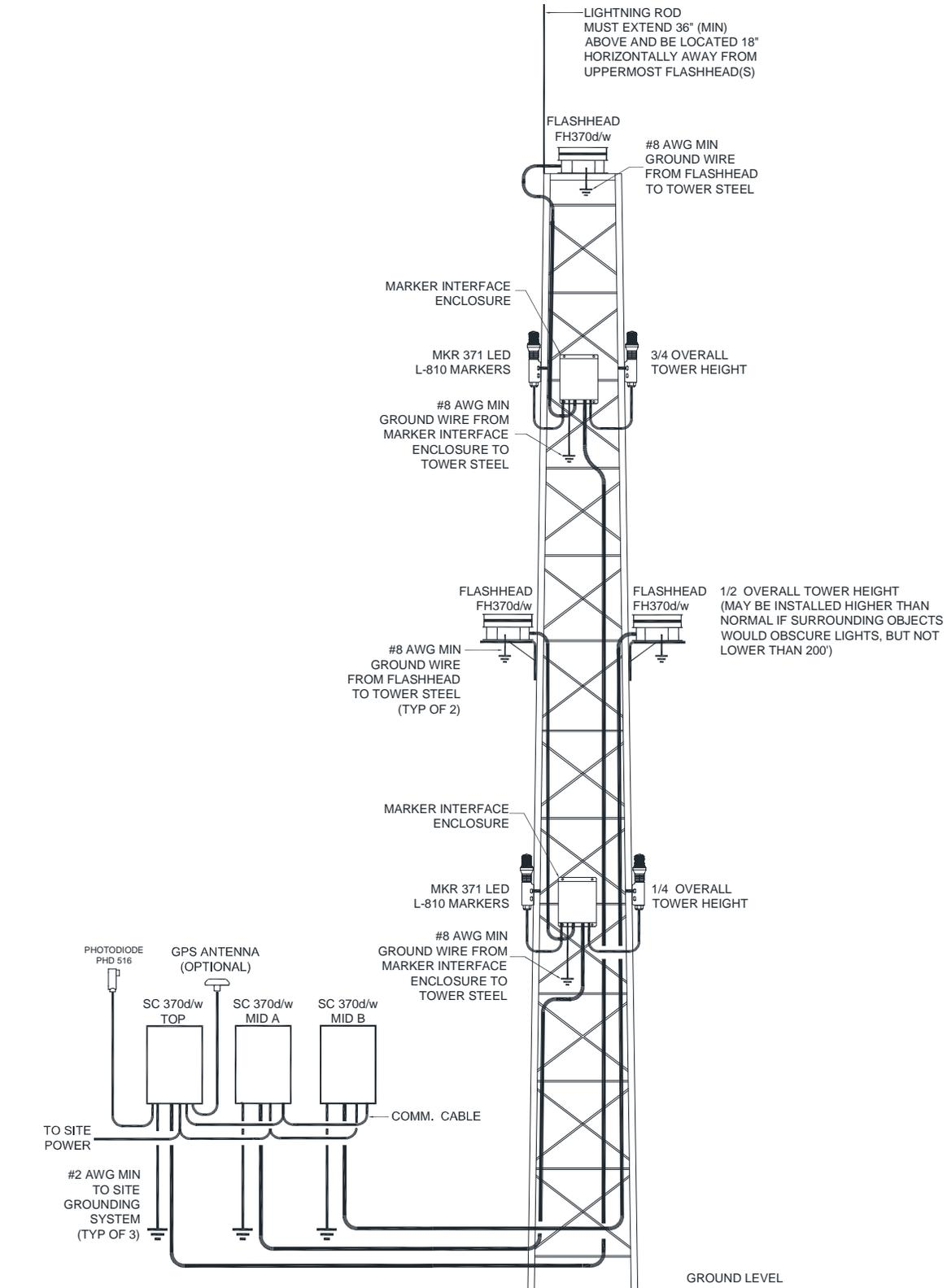
**Note:** Markers and Marker Interface Enclosure are omitted for D2 Installation and for version AC 70/7460-1L filed structure that are over 350' but not more than 700'.
