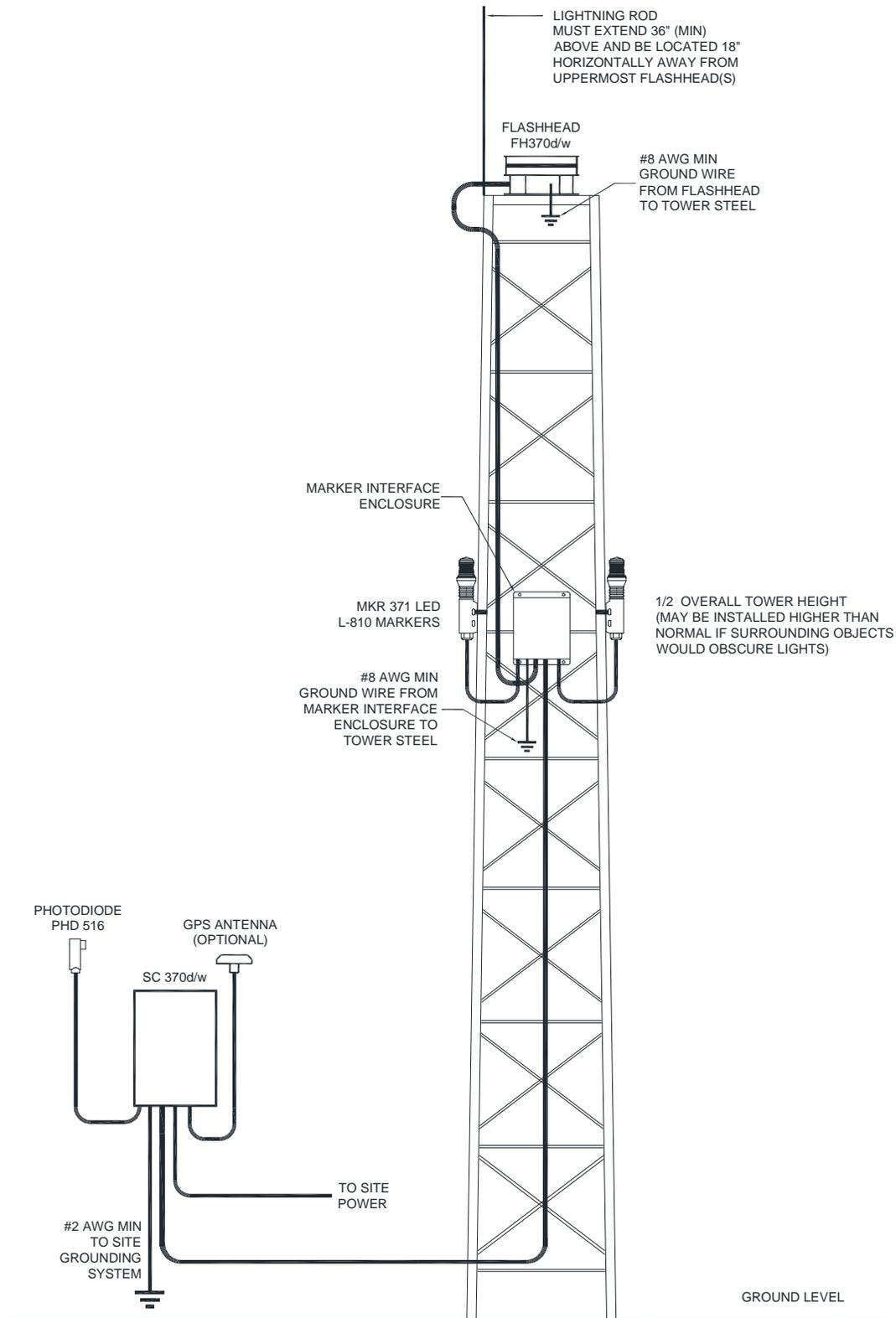
**Note:** Markers and Marker Interface Enclosure are omitted for D1 Installation and for version AC 70/7460-1L filed structure that are over 200' but not more than 350'.
