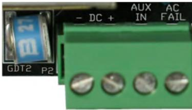
The Auxiliary Input (previously labeled LOW BAT) allows an external device, such as a radar system, to inhibit the output of the beacon. **Control via the Auxiliary Input is limited to systems consisting of a single SC 370 power and control unit.** Control is supplied by a dry contact from the external device connected to “Aux In” (P2 terminal 3) and “DC –” (P2 terminal 1). The fail-safe design requires a closed contact to inhibit the output of the beacon.
