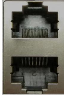
FTS 370 systems consisting of more than one SC 370 unit require connection of a communication cable between units. J4, located on the lower right of PCB1, provides connection for two RJ 45 connectors. The double RJ 45 connector allows the communication cables to be daisy chained from System 1 to each subordinate unit. Either port may be utilized as an input to or output from PCB 1. See “Communication Cable Kit” in Section 2 for additional connection and cable routing information.
