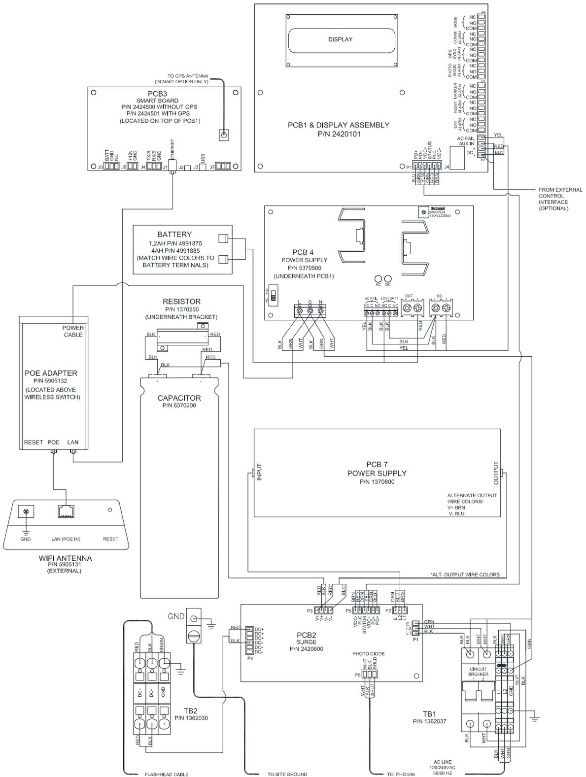
Figure 2-28 – SC 370 (AC) Internal Wiring with Wi-Fi Option
