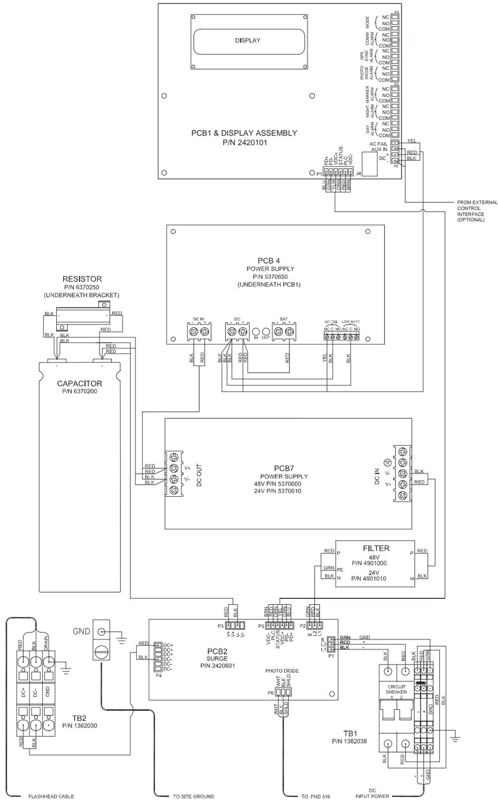
Figure 2-29 – SC 370 (DC) Internal Wiring Standard System
