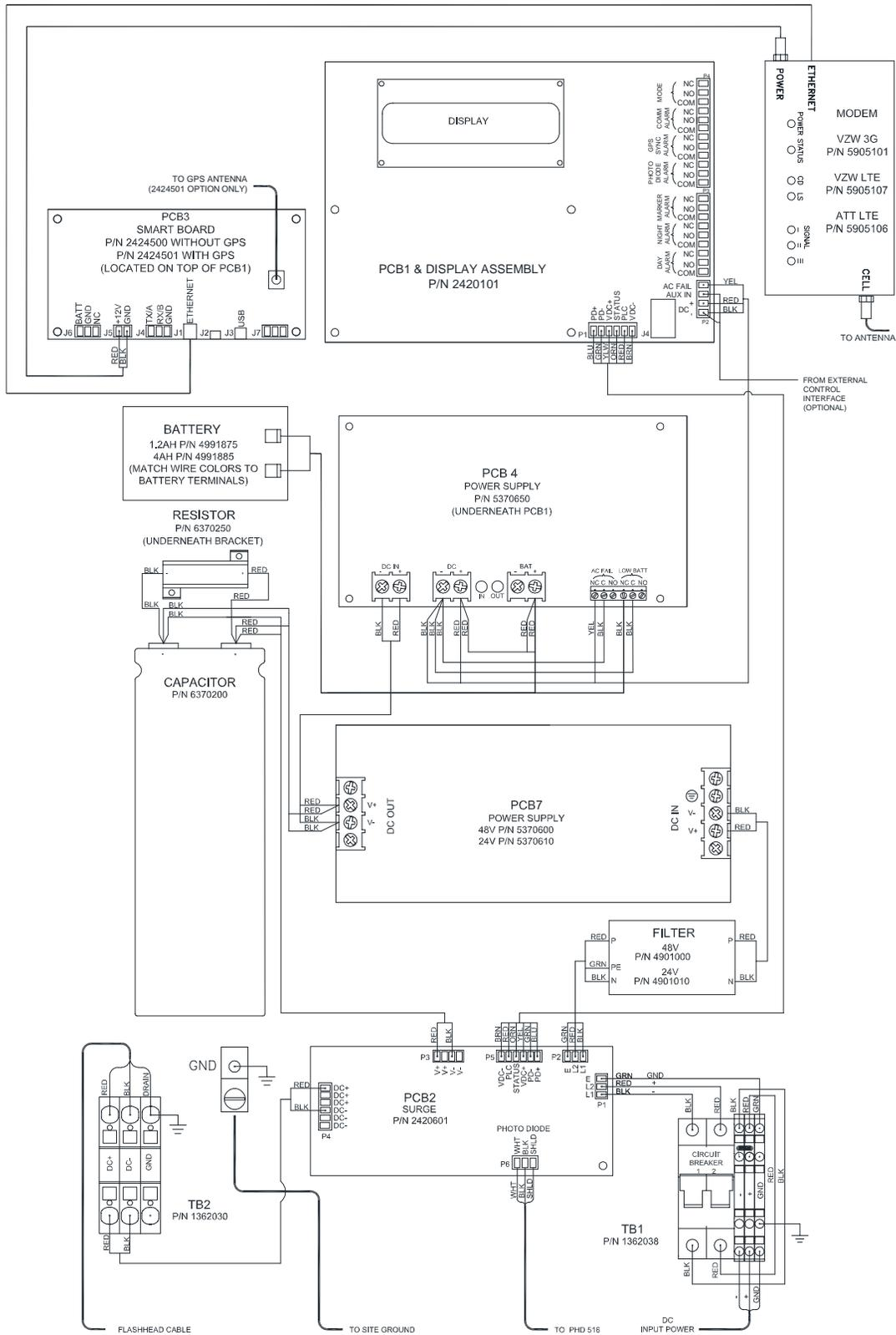
Figure 2-31 – SC 370 (DC) Internal Wiring with Modem Option
