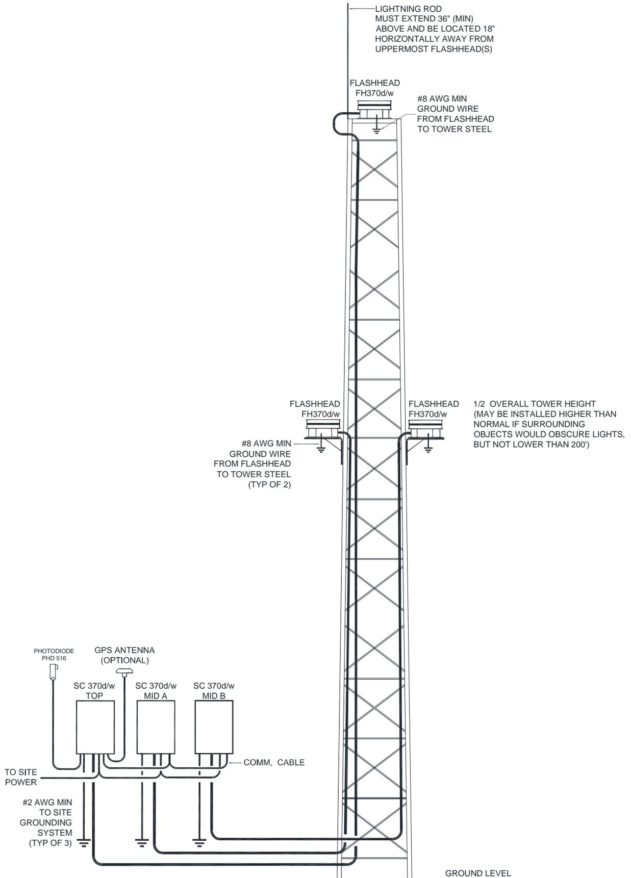
Figure 2-19 – Typical E2/D2 Avian Component Locations (AC 70/7460-1L)
