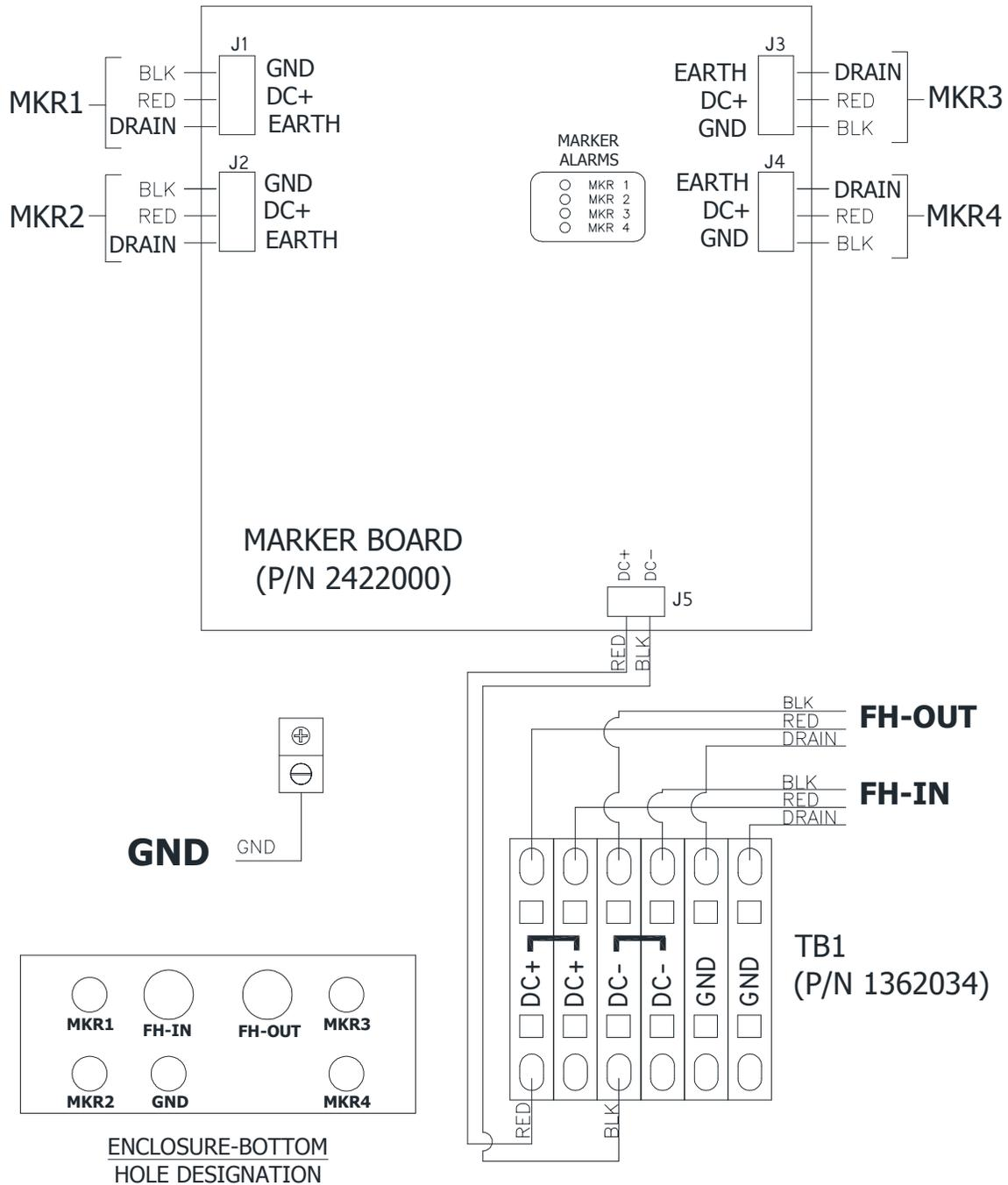
Figure 2-32 – Marker Interface Enclosure Wiring Diagram
