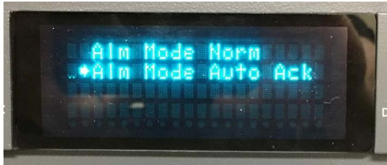
To change, use the Up button to move the arrow to the first option of "**Alm Mode Norm**".
