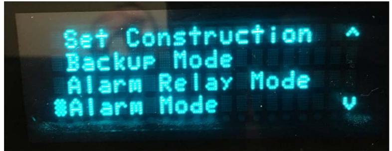
If the controller is set to Auto Acknowledge, it will be indicated by the presence of an arrow to the left of the second option, "**Alm Mode Auto Ack**".
