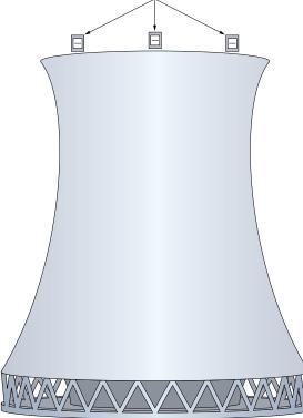
The number of light units recommended depends on the diameter of the structure
