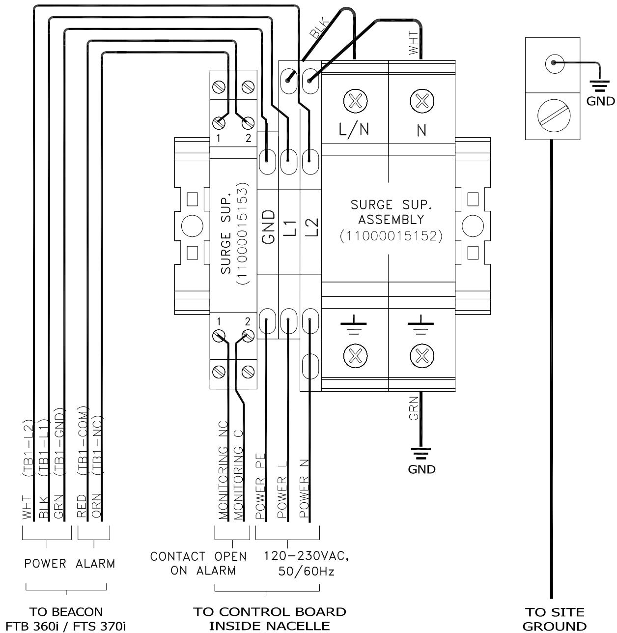
Figure 2-1 – OVP Internal Wiring
