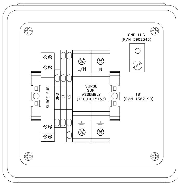
Figure 4-1 – OVP Component Locations
