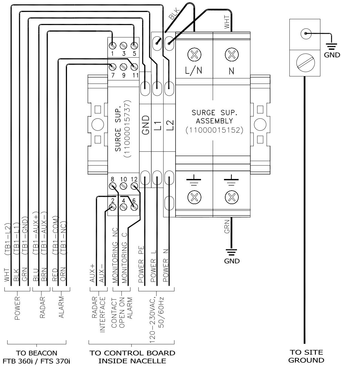
Figure 2-3 – OVP-RADAR Internal Wiring
