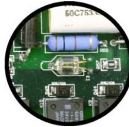
The trigger voltage neon provides an indication that trigger power is being supplied to the 2903800.
