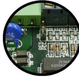
The RES PEC jumper is removed by default. The FTB 324 uses a PEC 510 resistive photocell for determining mode transition. To use an AC photocell, short this jumper and connect the output of the photocell to pins 4 (AC) and 5 (Return) of J5.
