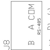
When all switches are OFF, the RS-485 is disabled. Once addressed, modem and RS-232 communication will be disabled and the RS-485 will become active. Table 1-4 defines the RS 485 address setup.
