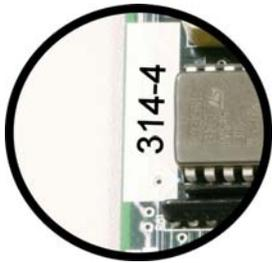
The 2903800 board is programmed from the manufacturer for operation in the PC 314-4. The board will be clearly marked in the area shown in Figure 1-2.
