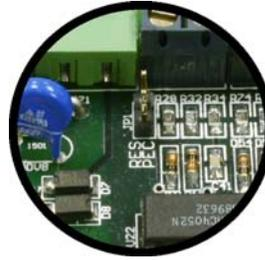
The RES PEC jumper is removed by default. The FTB 314-4 uses a PEC 510 resistive photocell for determining mode transition. To use an AC photocell, short this jumper and connect the output of the photocell to pins 4 (AC) and 5 (Return) of J5.
