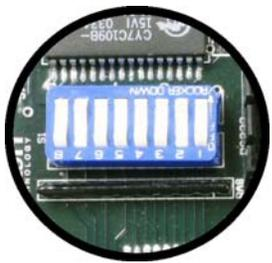
The options switch allows configuration of the RS-485 address, number of markers and alarm isolation.
