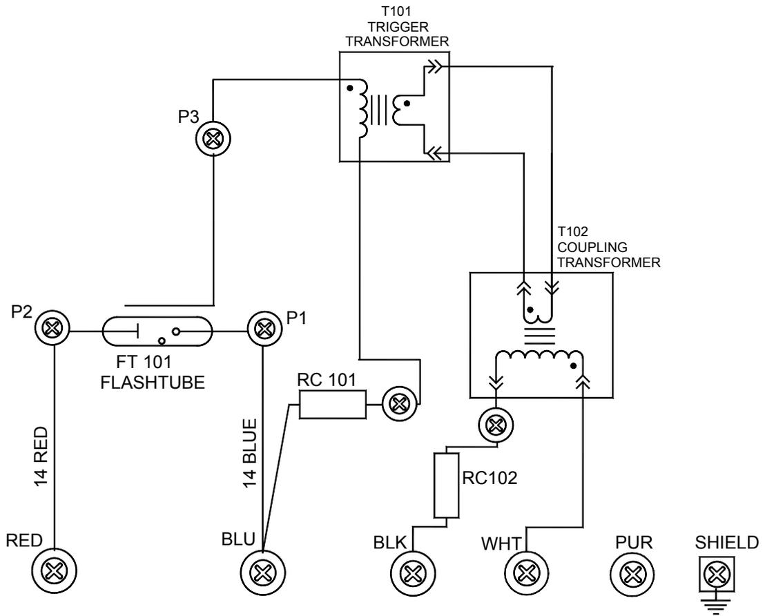
Figure 2-9 – FH 307 Internal Wiring
