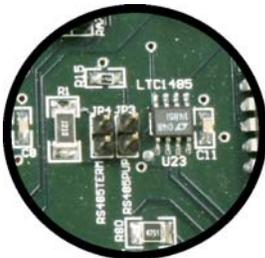
RS485TERM and RS485PUP are open by default and should be shorted only on the last 2903800 board in the series of equipment connected to an FTM-5000 or an FTW 17X series monitoring unit.
