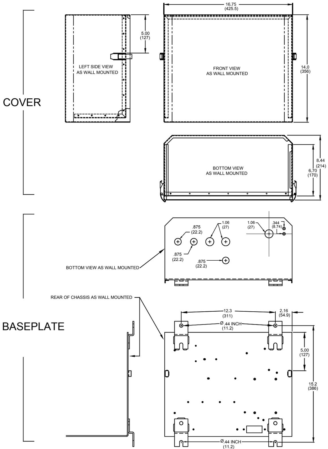
Figure 2-1 – Power Converter Mounting and Outline
