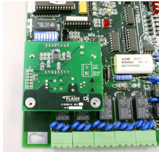
The terminal block can be removed for easy connection of the phone wires.
