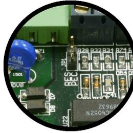
The RES PEC jumper is removed by default. The FTB 312-4 uses a PEC 510 resistive photocell for determining mode transition. To use an AC photocell, short this jumper and connect the output of the photocell to pins 4 (AC) and 5 (Return) of J5.
