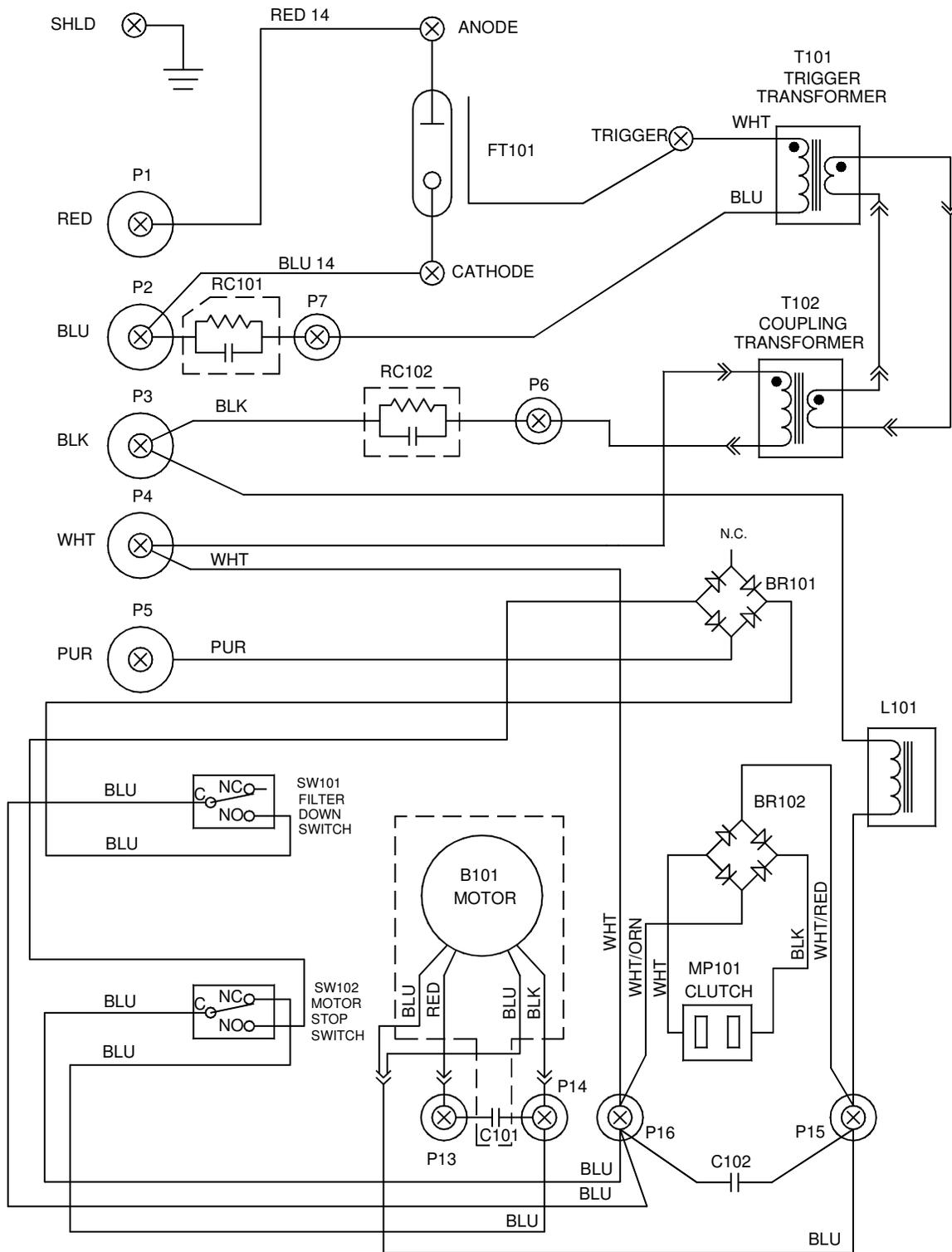
Figure 2-9 – FH 306 Internal Wiring
