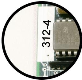
The 2903800 board is programmed from the manufacturer for operation in the PC 312-4. The board will be clearly marked in the area shown in Figure 1-2.
