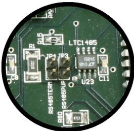
RS485TERM and RS485PUP are open by default and should be shorted only on the last 2903800 board in the series of equipment connected to an FTM-5000 as shown in Figure 2-10.
