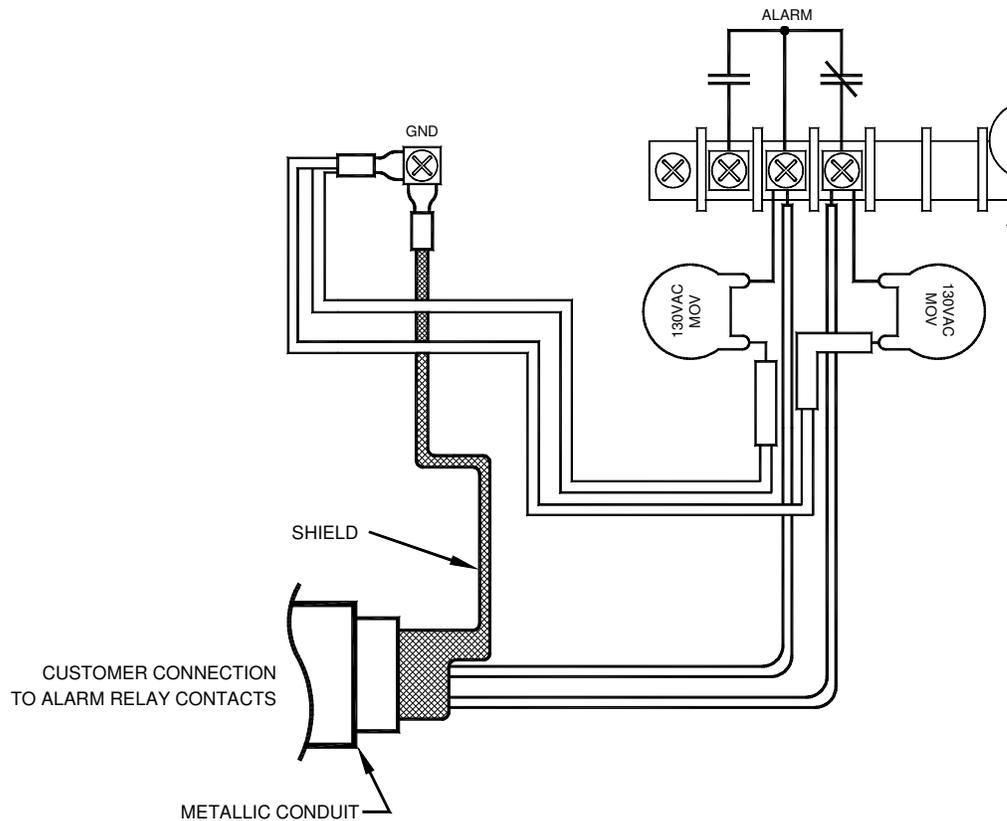
FLASH TECHNOLOGY ALARM RELAY CONTACTS ARE PROTECTED FROM VOLTAGE TRANSIENTS OF UP TO 1000 VOLTS. HOWEVER, WIRED ALARM CONTACTS CAN BE SUBJECTED TO VOLTAGES GREATER THAN 1000 VOLTS BECAUSE OF LIGHTNING. THE FOLLOWING RECOMMENDATIONS MINIMIZE THE POSSIBILITY OF DAMAGE CAUSED BY HIGH VOLTAGE TRANSIENTS ON THE ALARM RELAY CONTACTS OF FLASH TECHNOLOGY POWER CONVERTERS.
