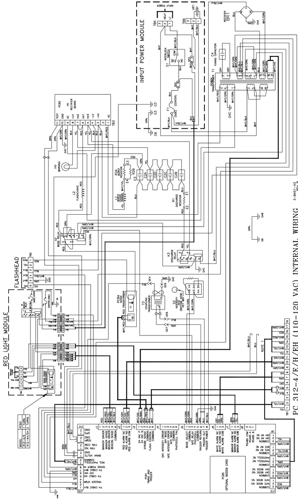
Figure 2-6 – PC 312-4 Power Converter Internal Wiring (110-120V)
