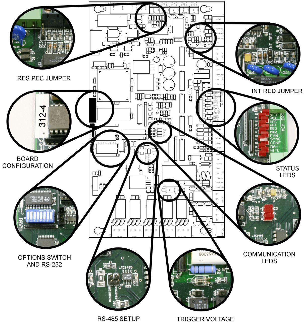
Figure 1-2 – 2903800 Board Configuration
