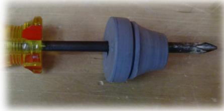
2. Feed the cable through the gray cord grip (The cable will create a larger opening and will ensure it is the appropriate size).
